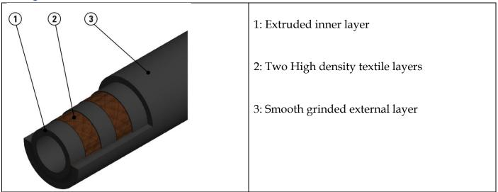
The pump hose liner material should be chemically resistant with the product to be pumped. Dependent on the specific requirements of your application a corresponding pump hose must be selected. For each pump model various hose types are available. The material of the inner liner of the pump hose determines the hose type. Each hose type is marked by a unique colour code.
